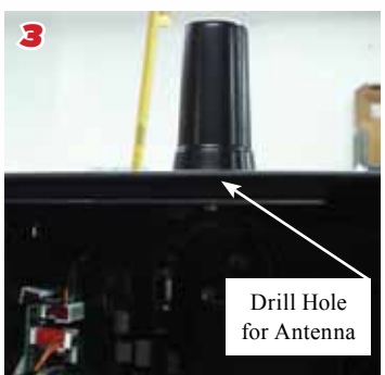
Step 3 Drill a hole in the top of the machine to mount the antenna using a 5/8th inch steel hole saw.
