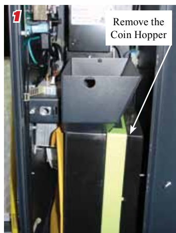
Step 1 Remove the Coin Hopper(s) from the machine.
